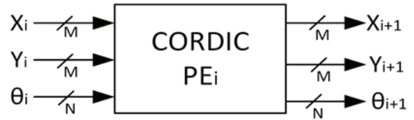
Figure 2: Standard CORDIC Processing Element (PE)
