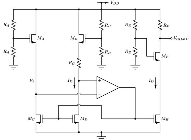
**Figure 2:** Compensation circuit
