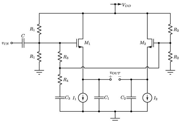
**Figure 1:** RF power detector core schematics
