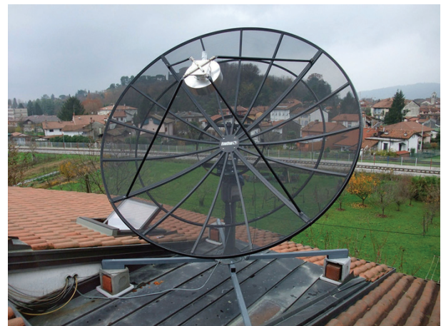
Figure 2: Mesh reflector with feed, LNA and azimuth/elevation positioner.
