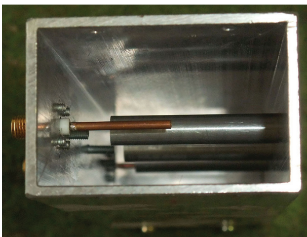
Figure 11: Inside the comb-filter cavity.
