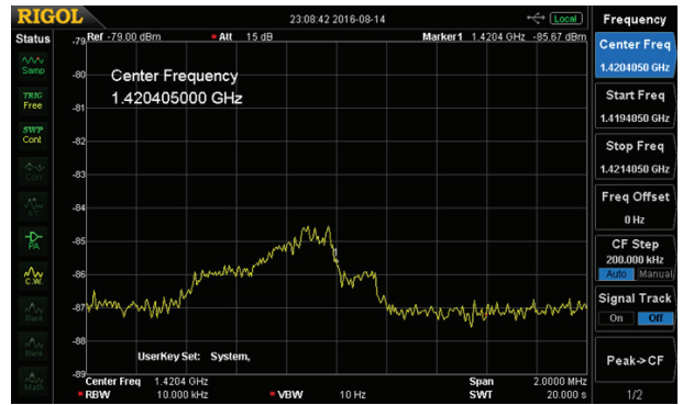
Figure 18: Neutral-hydrogen spectrum from the direction of the star \alpha Scutum.
